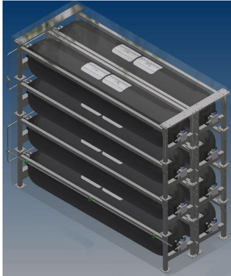
Figure 43: Representative integration of H 2 storage system in the technical carriage. Source: CAF
