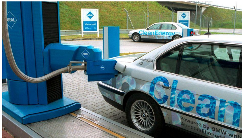
Figure 15: Automatic LH 2 refuelling system at Munich Airport [22]
