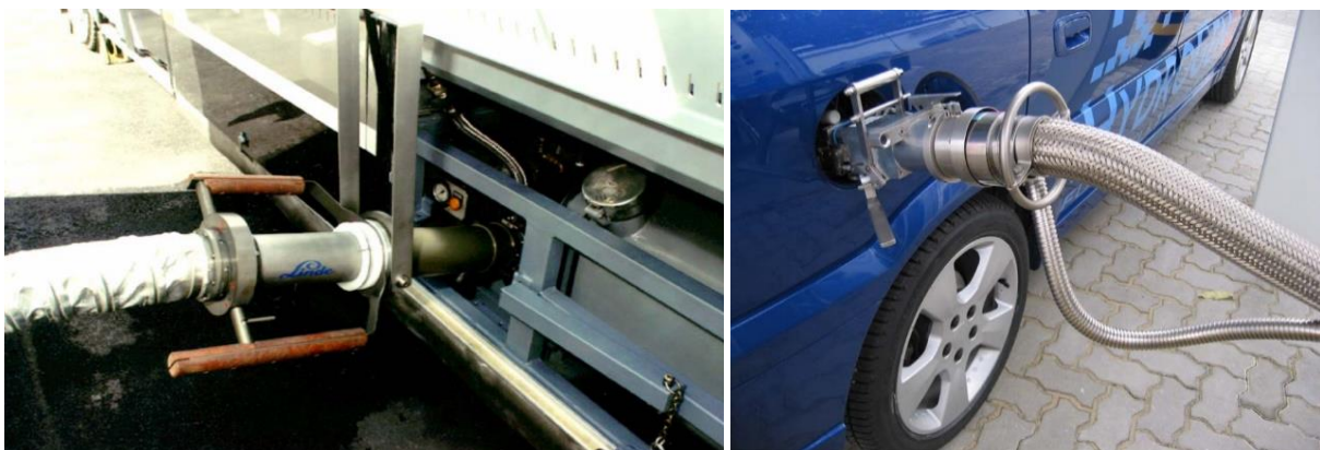
Figure 14: LH 2 fuelling nozzles of the first generation in 1994 (left) and second generation in 1999 (right) [21]
