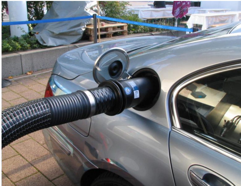
Figure 17: The LH 2 quick-connect refuelling nozzle [24]
